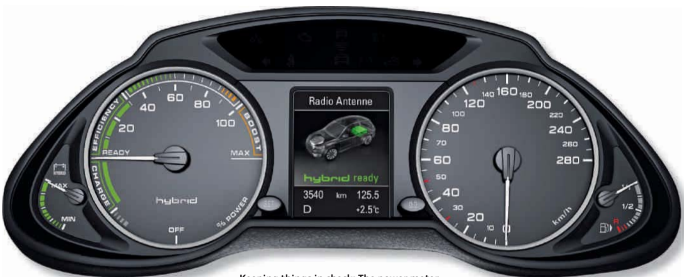
Keeping things in check: The power meter (left) and the display in the middle make the various driving modes of the hybrid drive transparent and show the power flows.
