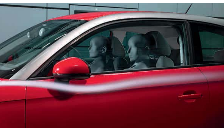
Acoustics test: Noises inside the car are measured using mannequins to which microphones have been attached.
