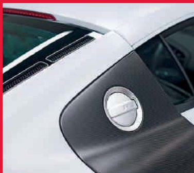
Visible high-tech: CFRP sideblade of the Audi R8 GT.
