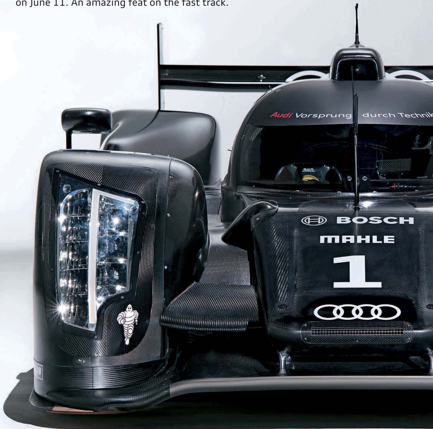
The Audi R18 is a new development: the carbon-fiber chassis, innovative LED lighting technology – and a roof.
