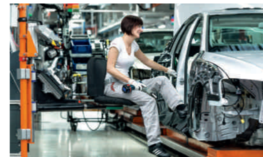
Impressions from the production shop: Sabine Wittmann checks the strength of the body-in-white spot welds with an ultrasonic device (top left). Factory tour guide Sabine Mayer explains how a car's body is built (top right). Simone Rehm uses the ergonomic assembly seat when installing the roof module (below, center).
