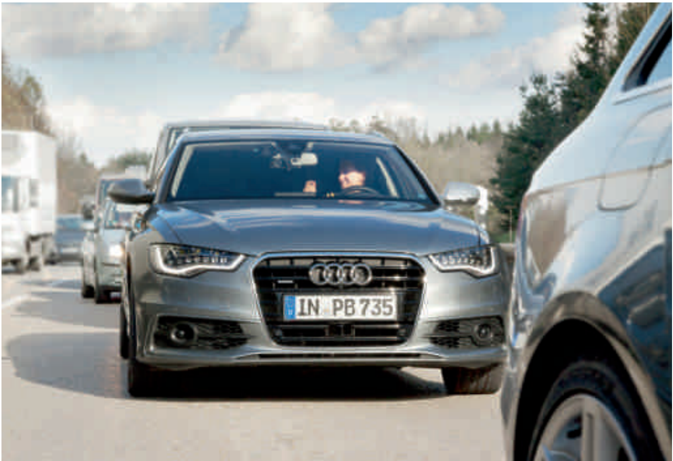
Piloted driving in traffic: progress through cutting-edge technology. Scanning distances, accelerating, braking and staying in lane. To enable piloted driving, Audi uses multiple redundancy to assess the driving situation. The exterior sensors consist of a dual radar system, a laser rangefinder and cameras.
