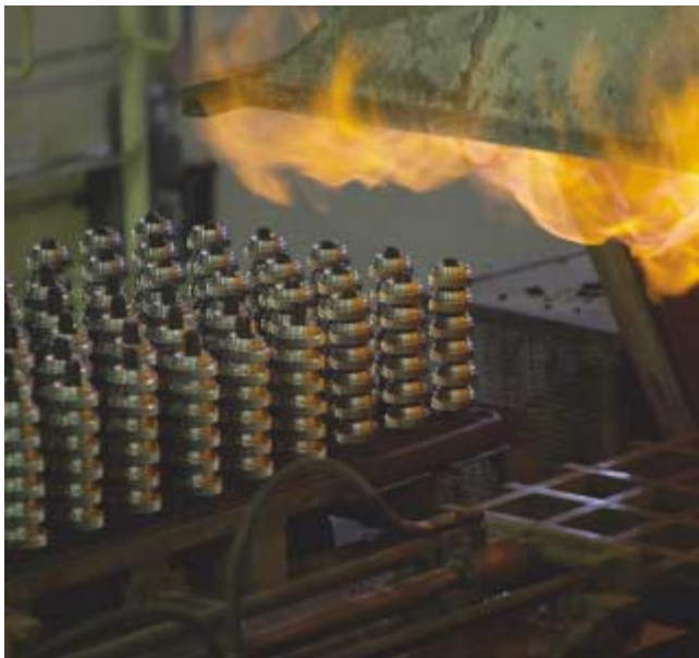
Heat treatment of gears at the Seville plant in Spain.
