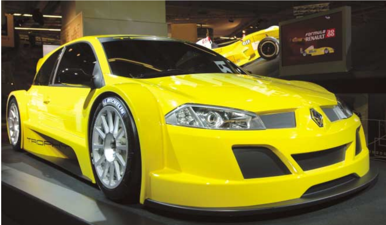
Set to fly Renault's colors on the track — Mégane Trophy weighs in at around 950kg and has a 3.5-liter 24V V6 engine developing over 320hp connected to a semi-automatic six-speed gearbox.
