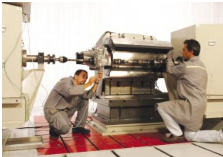
An acyclic drivetrain test bed, the first of its kind in Europe, helps the NVH unit correct undesirable vibro-acoustic features.
