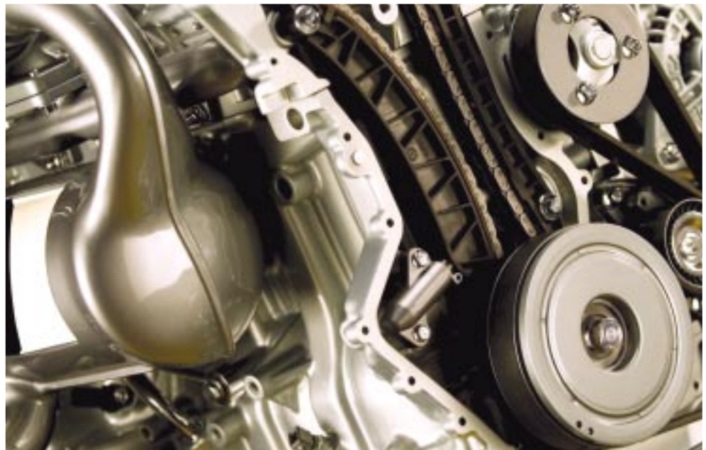
The 175hp version of the 2.0 dCi, fitted with a periodic-regeneration particulate filter, offers the highest power output in its class.
