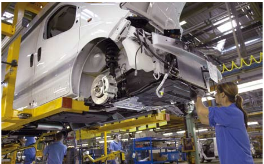
Production of Renault Traffic cross-badged as Nissan Primastar in Nissan's plant in Barcelona, Spain.
