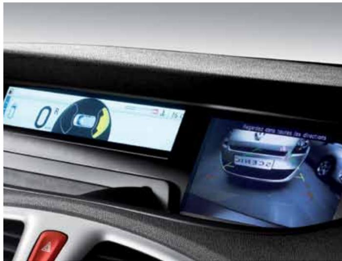
To make parking maneuvers easier and safer, the reversing camera projects a picture of the area behind the car onto the navigation screen.
