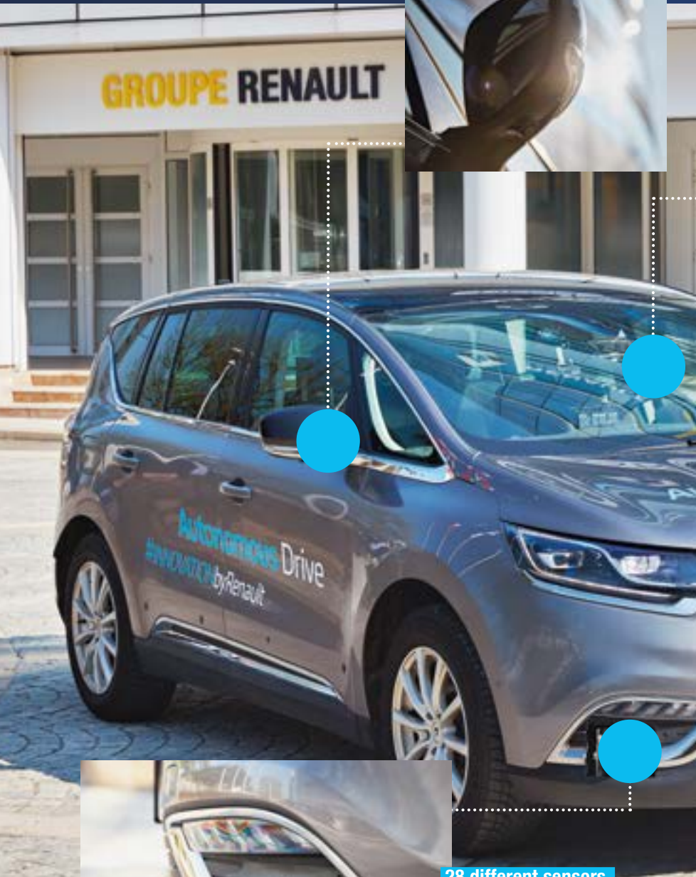
28 different sensors, corner radars, a long-range central radar and LIDARs are part of the range of sensors found on the autonomous Espace.
