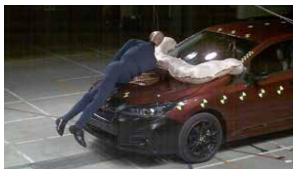
Collision tests of the first vehicle in Japan equipped with a pedestrian protection airbag
